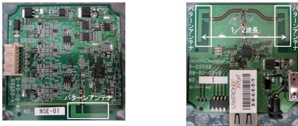
図4 Gen.2の子機(左)および親機(右)の基板 Figure 4 Photographs of wireless slave monitoring device (left) and master monitoring device (right)
