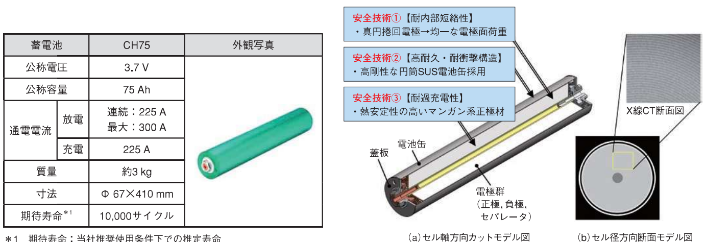
図12 CH75電池の概要 Figure 12 Specifications, appearance and safety technologies of lithium-ion battery CH75 cell
