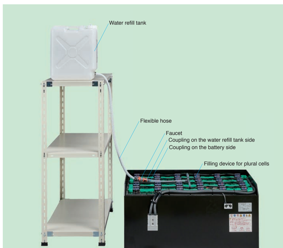
Start of water refilling: Opening the faucet automatically starts refilling water into all batteries (be sure to open the faucet fully).
